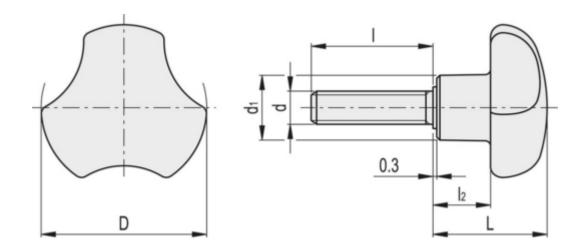
$\begin{array}{lll} D & = 25 \\ d1 & = 12 \\ Dg & = - \\ I2 & = 10 \\ L & = 20 \\ L1 & = 16 \\ Weight in (g) = 9 \end{array}$
